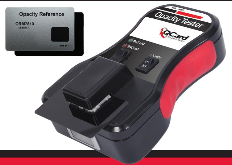
The Q-Card opacity tester is designed as a go/no-go opacity test for ISO and MasterCard CQM standards. To test a card, the unit utilizes a calibration card to establish the baseline opacity criteria. The card under test will be evaluated against the baseline criteria, if the displayed value is less than or equal to the baseline, the card will pass.
